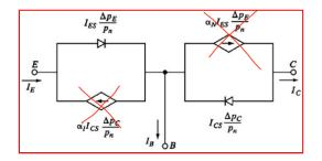
(c) <u>TRUE</u> or FALSE : The current sources represent a diode that is reversed biased, and simply capturing current sent to it across the base from a diode that is forward biased.
